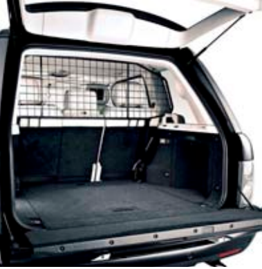
Cargo Barrier Half Height VUB0002120 Easily removed. Retains cargo according to EC regulation 17.
